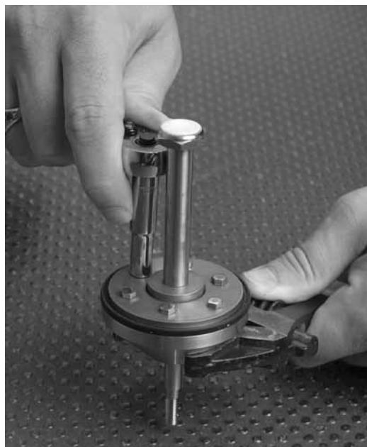
Figure 3. Use Spring Seat (Key 4) and Stem Assembly (Key 2) to Align Disc Retainer (Key 8)
