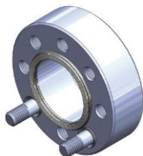
Placement of Spiral-Wound Gasket
