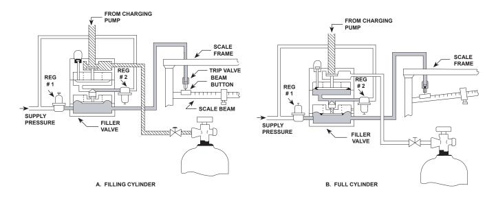
Figure 2. Operational Schematic
