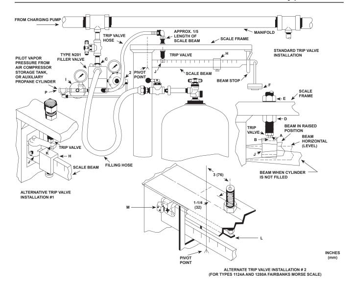
Figure 3. Type N201 Installation
