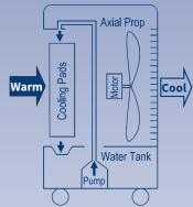
Water from an onboard tank is pumped to the top of a filterlike cooling pad. Then, a 3100 CFM fan pulls warm, environmental air over the filter and pushes out air with a cooling effect 30+ feet.
